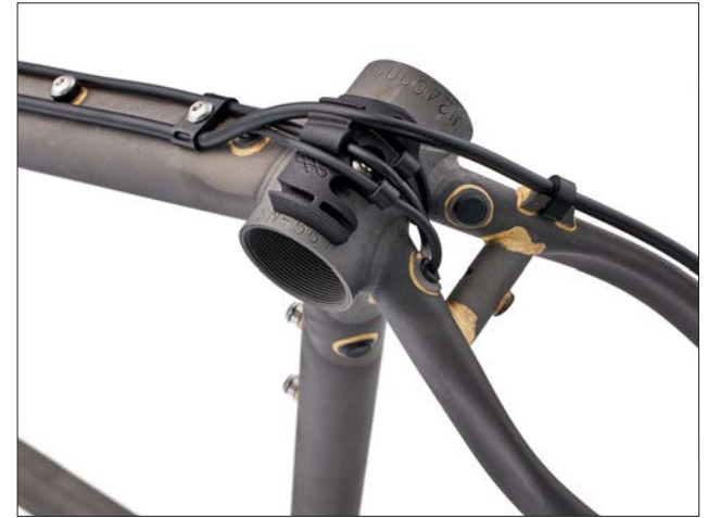
Alternative orientation for UK / Aus / NZ / Jpn. Rear brake on left side of handlebar. Rear light on drive side dropout.
