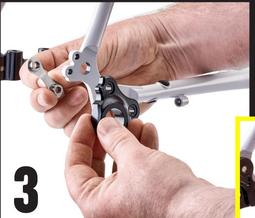
**3 & 4** - Unlike the other inserts, the T-Type piece fits to the outside face of the dropout. The bolts screw into a stainless threaded plate which is mounted to the inside face. The male mating parts of both pieces should fit snugly into the holes in the dropout face.
