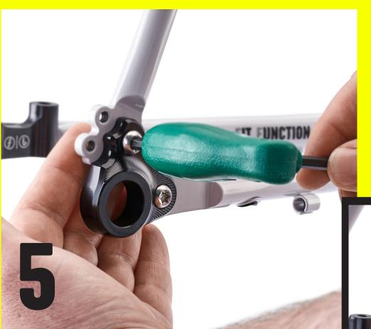
**5** - Add the T3O 12mm bolts and **torque both bolts to 8 Nm.**
